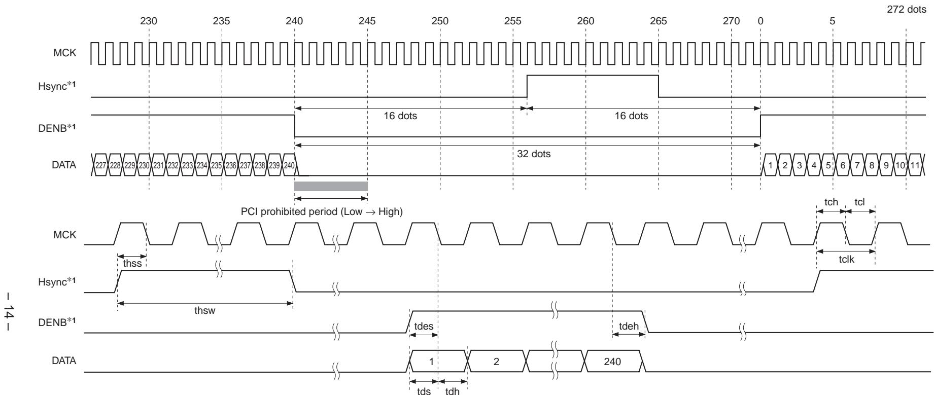
\*1 Input either Hsync + Vsync or DENB as sync input signal.
