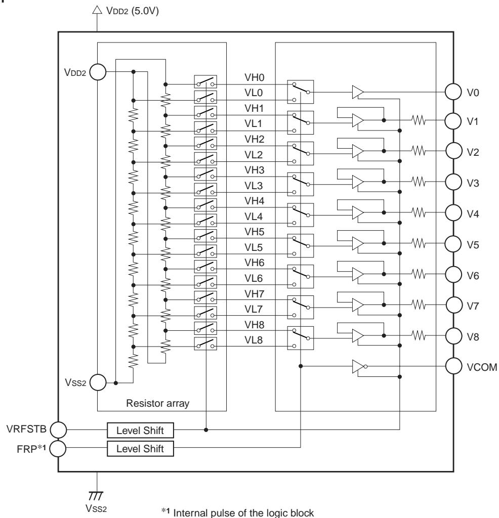
**Electrical Characteristics (Reference voltage driver block)****Resistor array output voltage**(V<sub>DD1</sub> = 3.3V, V<sub>DD2</sub> = 5.0V, Ta = 25°C)
