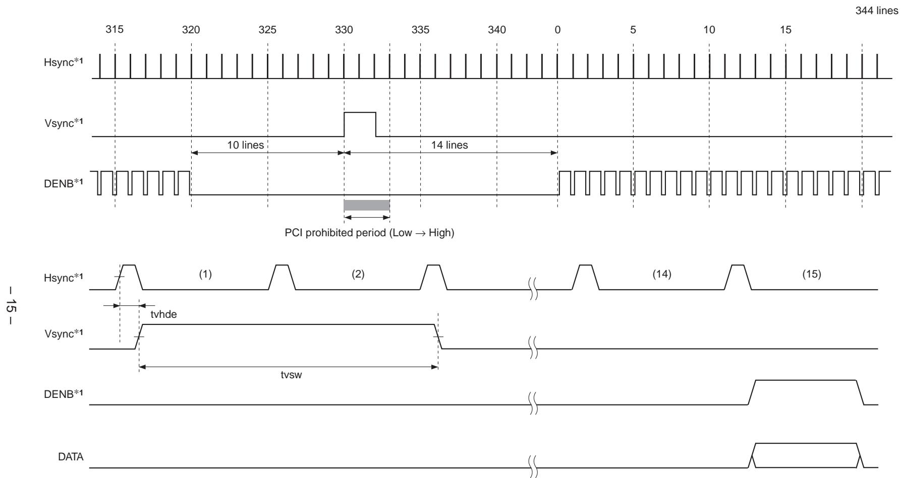
\*1 Input either Hsync + Vsync or DENB as sync input signal.
