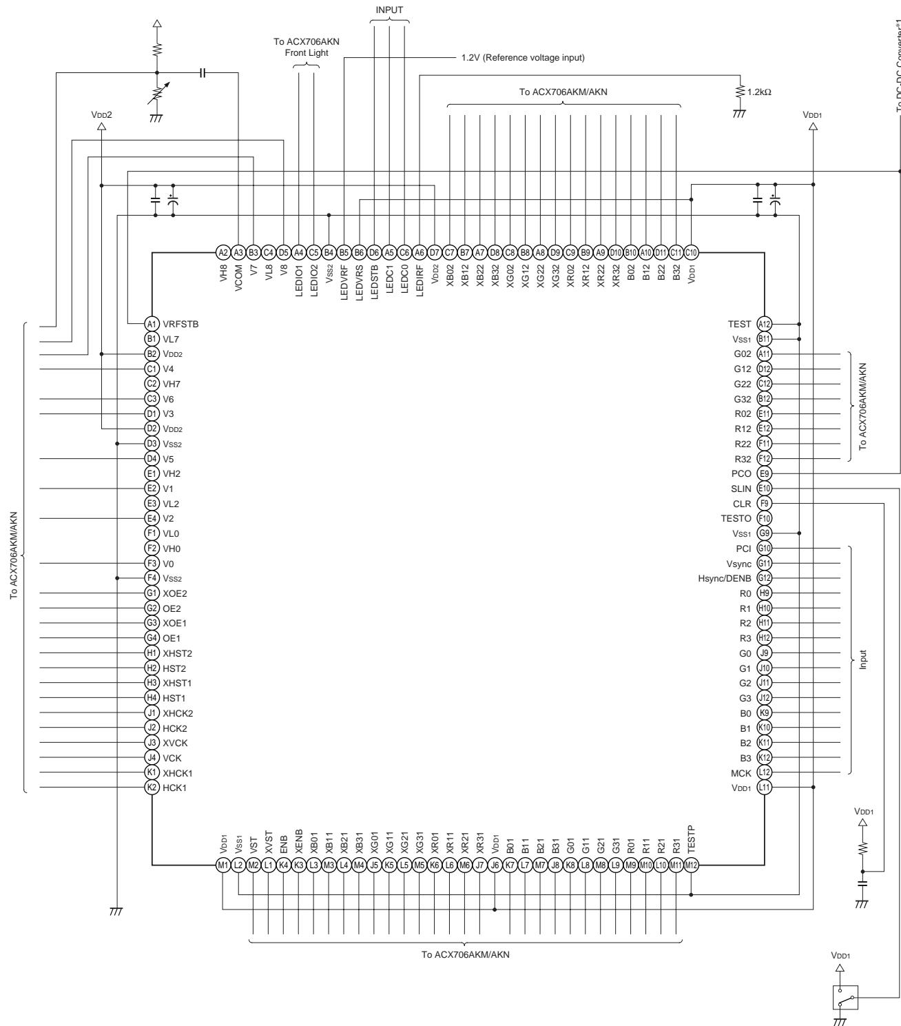
\*1 Connect PCO to DC-DC converter that can control power on/off of the ACX706AKM/AKN.
