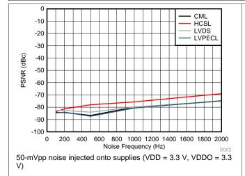
Figure 13. PSNR vs. Noise Frequency (50 mVpp) For 156.25-MHz Output
