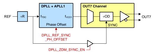
Figure 52. DPLL ZDM Synchronization Between Reference Input and OUT7
