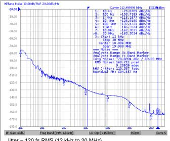
Jitter = 120 fs RMS (12 kHz to 20 MHz) DPLL Mode With Cascaded APLL2  $f_{VCO2} = 5737.5 \text{ MHz}$
