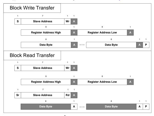
Figure 59. I<sup>2</sup>C Block Register Transfers
