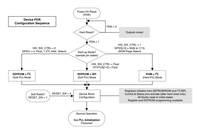
Figure 53. Device POR Configuration Sequence
