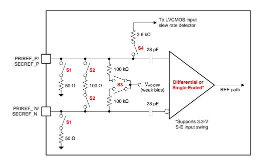
Figure 28. Reference Input Buffer
