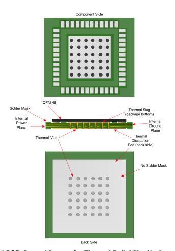
Figure 68. General PCB Ground Layout for Thermal Reliability (8+ Layers Recommended)
