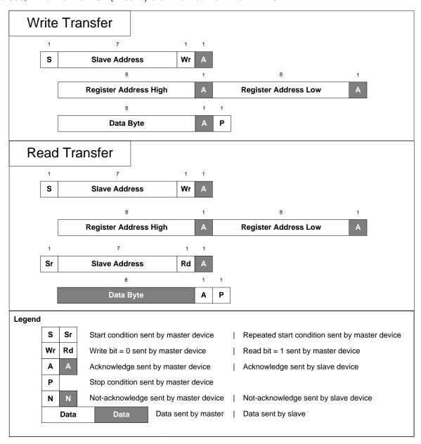
Figure 58. I<sup>2</sup>C Byte Write and Read Transfers
