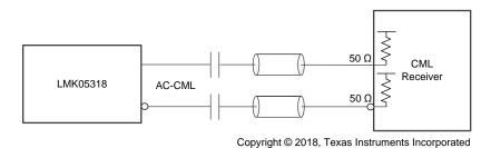
Figure 49. AC-CML Output to CML Receiver With Internal Termination/Biasing
