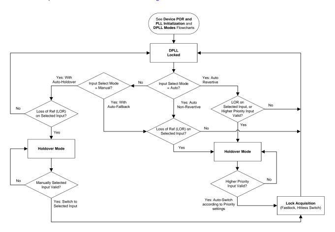
Figure 36. Reference Input Selection Flowchart
