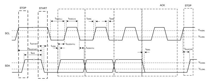
Figure 3. I<sup>2</sup>C Timing Diagram
