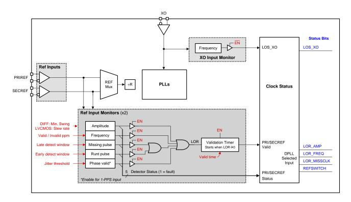
Figure 37. Clock Monitors for Reference and XO Inputs
