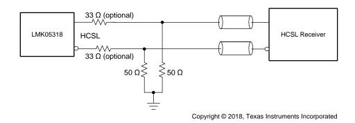
If HCSL Internal Termination (50- $\Omega$  to GND) is enabled, short 33- $\Omega$  and remove 50- $\Omega$  external resistors.
