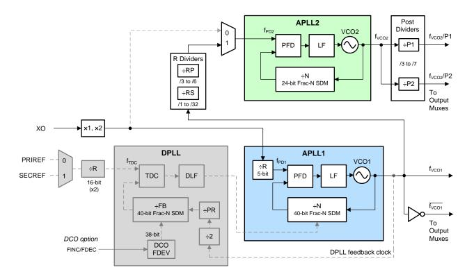
Figure 26. APLL-Only Mode With Cascaded APLL2
