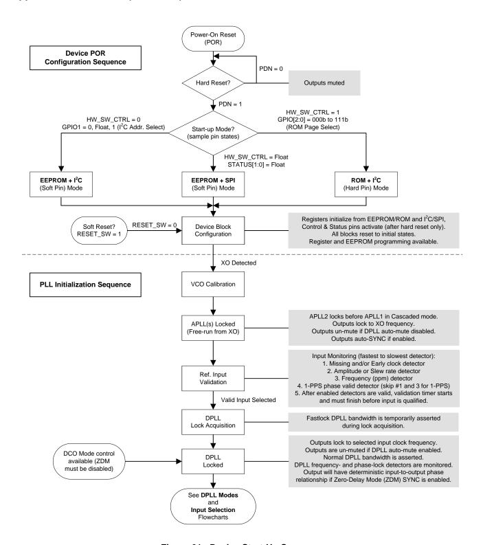
Figure 61. Device Start-Up Sequence
