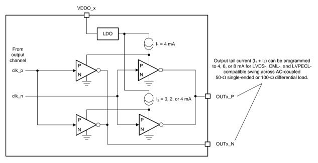
Figure 46. AC-LVDS/CML/LVPECL Output Driver Structure
