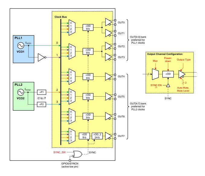
Figure 45. Output Clock Distribution
