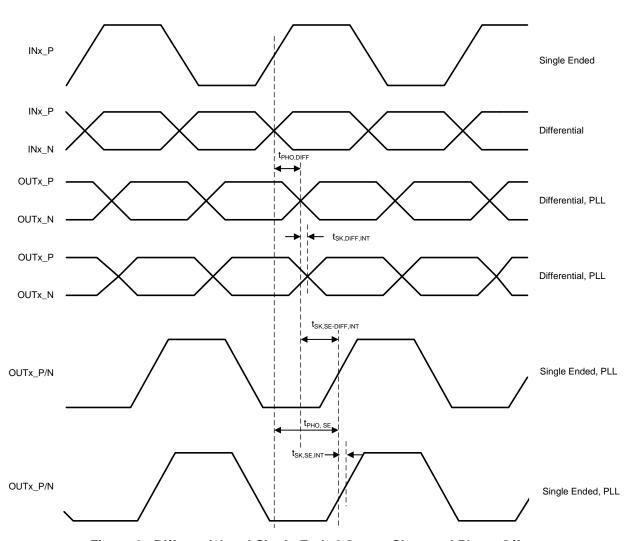
Figure 6. Differential and Single-Ended Output Skew and Phase Offset
