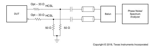
Figure 20. HCSL Output Phase Noise Test Configuration
