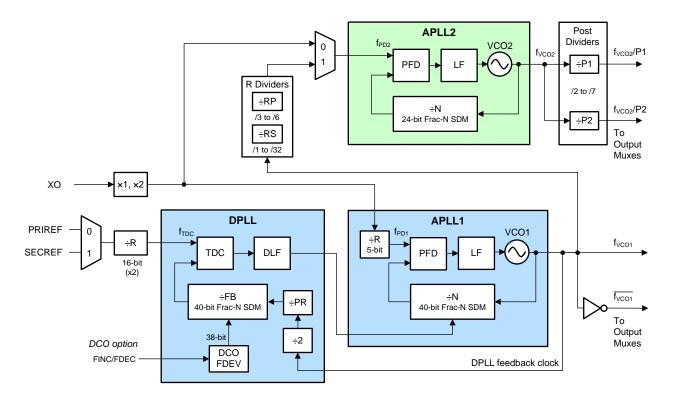
(1) DCO frequency adjustments can be software or pin controlled.
