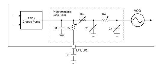
Figure 44. Loop Filter Structure of Each APLL
