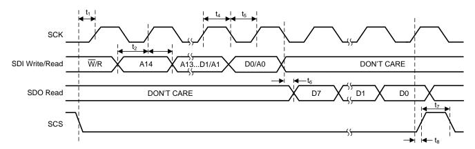
Figure 2. SPI Timing Parameters
