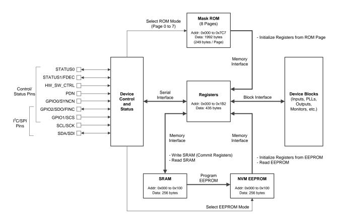
Figure 57. Device Control, Register, and Memory Interfaces
