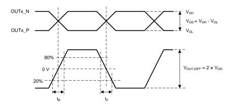
Figure 4. Differential Output Voltage and Rise/Fall Time
