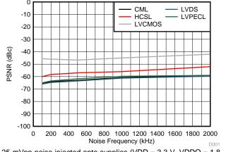
25-mVpp noise injected onto supplies (VDD = 3.3 V, VDDO = 1.8
