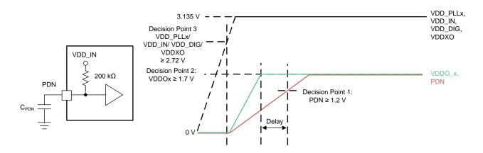
Figure 63. Recommendation for Power Up From Split-Supply Rails
