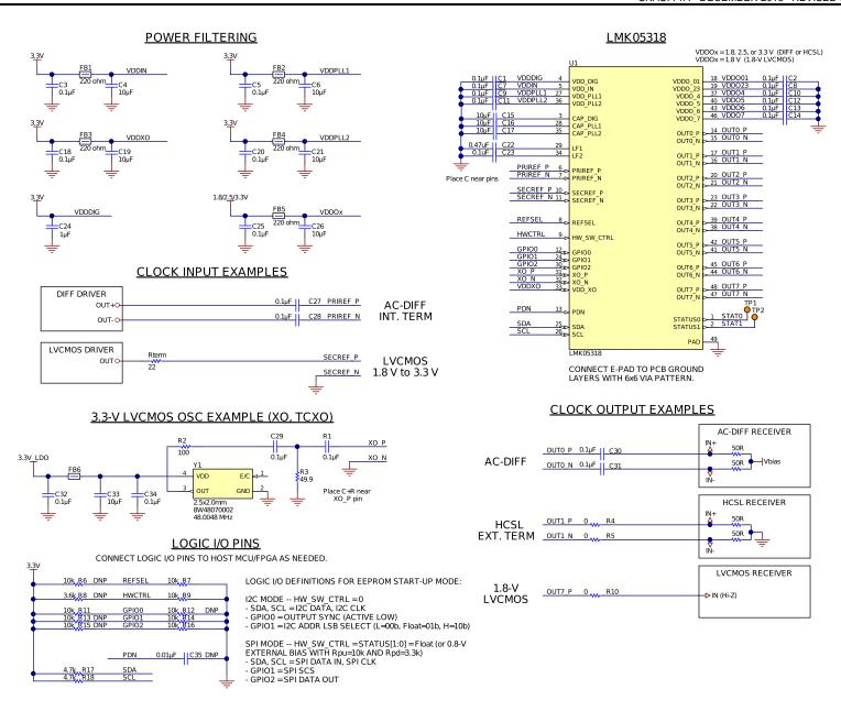
Figure 64. LMK05318 Reference Schematic Example
