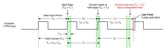
Figure 39. 1-PPS Input Window Detector Example
