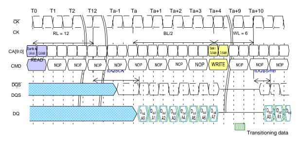
The minimum time from the burst READ command to the burst WRITE command is defined by the read latency (RL) and the burst length (BL). Minimum READ-to-WRITE latency is RL + RU(tDQSCK(MAX)/tCK) + BL/2 + 1 - WL clock cycles.
