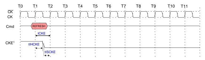
${\tt NOTE~1} \quad {\tt CKE~can~go~LOW~tIHCKE~after~the~clock~on~which~the~REFRESH~command~is~registered}.$
