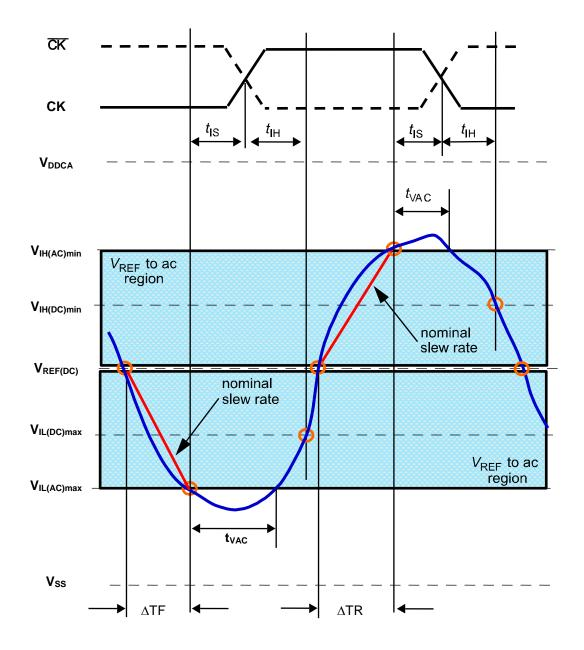
$$\begin{array}{ll} \text{Setup Slew Rate} = \frac{V_{\text{REF(dc)}} - V_{\text{IL(ac)}} \text{max}}{\Delta \text{TF}} & \text{Setup Slew Rate} = \frac{V_{\text{IH(ac)}} \text{min - } V_{\text{REF(dc)}}}{\Delta \text{TR}} \end{array}$$
