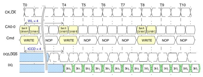
NOTE 1 The seamless burst WRITE operation is supported by enabling a write command every four clocks for BL = 8 operation.
