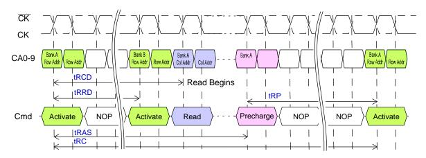
NOTE 1 A PRECHARGE-all command uses tRPab timing, while a single-bank PRECHARGE command uses tRPpb timing. In this figure, tRP is used to denote either an all-bank PRECHARGE or a single-bank PRECHARGE.
