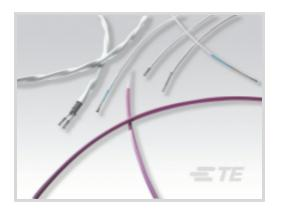
Cable Type: MIL-DTL-27500 Voltage Rating: 600 VAC Insulation Material: Modified Radiation Cross-linked ETFE Polymer Conductor Material: Silver-Coated Copper Wire Size: 14 AWG
