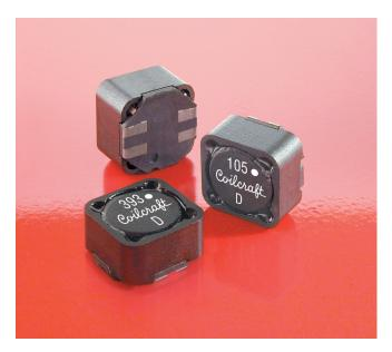
The ML612PND series of coupled inductors was designed for high temperature applications — up to  $155^{\circ}$ C. The excellent coupling coefficient (k  $\geq$  0.98) makes it ideal for use in SEPIC applications. In SEPIC topologies, the required inductance for each winding in a coupled inductor is half the value needed for two separate inductors, allowing selection of a part with lower DCR and higher current handling.
