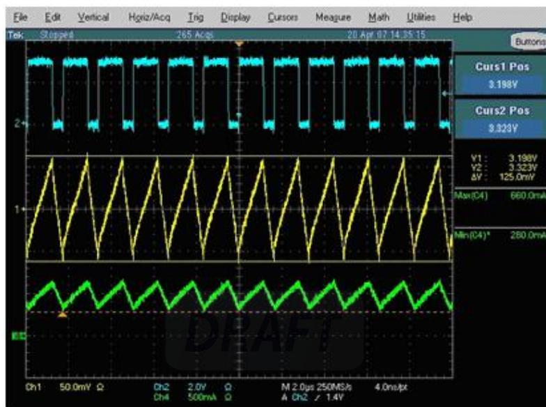
**Figure 20. Electrolytic 100 $\mu$ F (Ripple Too High)**
