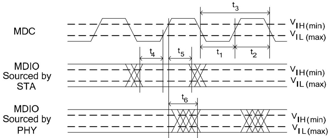
Figure 26. MDC/MDIO Management Timing Parameters
