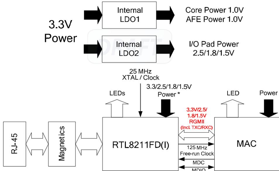
\*Note: 3.3/2.5/1.8/1.5V power here means I/O pad power sourced from external power; not from the internal LDO.
