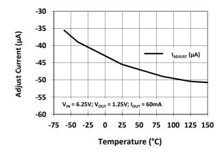
Figure 5 - Adjust Current vs. Temperature
