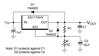
Figure 16 · Use of Protection Diodes
