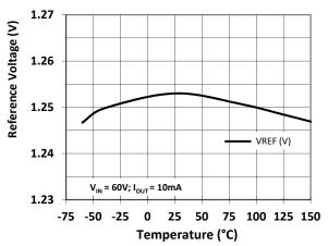
Figure 3 - Reference Voltage vs. Temperature
