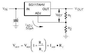
Figure 13 - Basic Regulator Circuit
