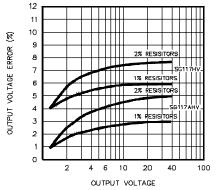
Figure 14 · Voltage Tolerance vs. Resistor Tolerance
