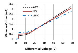
Figure 8 - Minimum Current vs. Input / Output Differential Voltage
