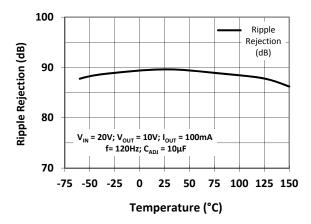
Figure 6 - Ripple Rejection vs. Temperature
