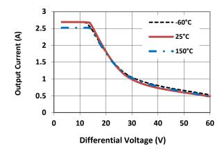
Figure 7 · Output Current vs. Input / Output Differential Voltage for K, P, G, IG Packages
