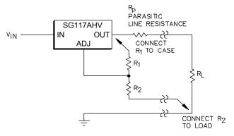
Figure 17 · Connections for Best Load Regulation
