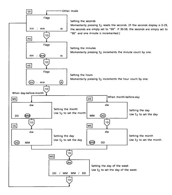
Note 16: In all setting states except for second reset, holding down S<sub>2</sub> automatically advances the count.
