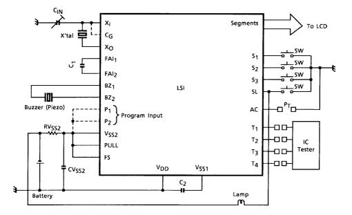
Note 19: For specifications featuring an alarm, add a transistor and buzzer.
