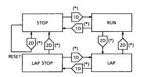
Note 10: All day of the week marks are lit, with the relevant mark brinking at 2 Hz depending on state. When the LAP display or the LAP STOP display are selected, the LAP sign flashes at 2 Hz and shows the lap time.
