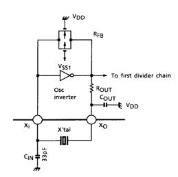
$f_{OSC} = 32.768 \text{ kHz}$ X'tal:  $R_S = 30 \text{ k}\Omega \text{ (max)}$
