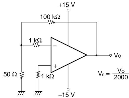
Figure2 Channel Separation Measurement Circuit
