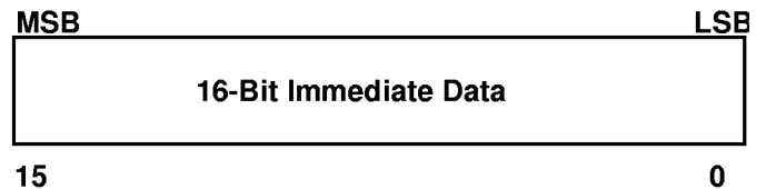
Figure 32c. Register Immediate Instruction Format
