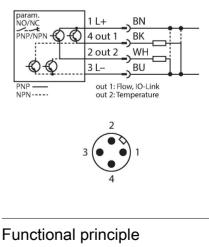
The flow sensor functions according to the calorimetric principle. The distinctive feature of this principle is that the flow rate correlates directly to the thermal loss of energy in the probe. The increased loss of energy is
