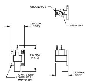
Dimensions in ( ) are in mm. Case is electrical ground.
