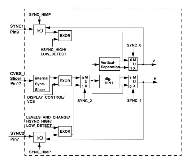
Figure: Signal-pathes of the sync-seperation-circuit
