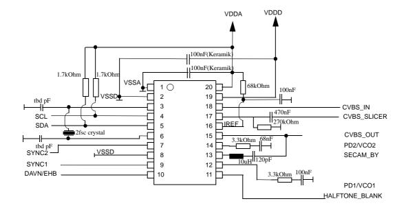
Environment for a system with 2fsc as external system-clock in oscillator-mode 11:
