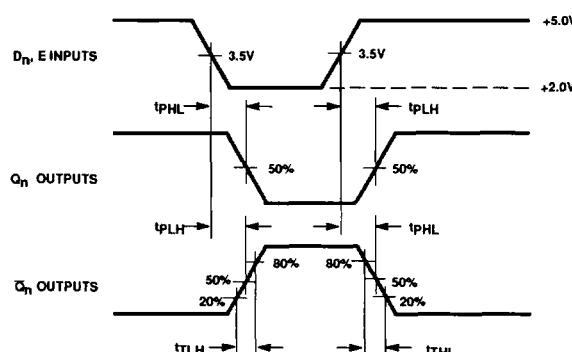
Waveform 1. Propagation Delay and Transition Times
