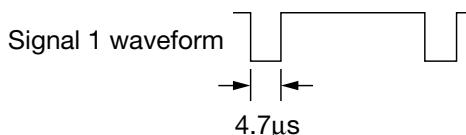
\*3 Measuring horizontal sync signal pull-in range
