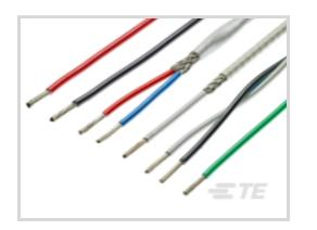
Cable Type: Spec 44 Voltage Rating: 600 VAC Insulation Material: Modified Radiation Cross-linked PVDF Conductor Material: Tin-Coated Copper Wire Size: 24 AWG
