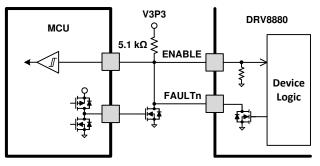
Figure 27. Methods For Operating in Retry Mode
