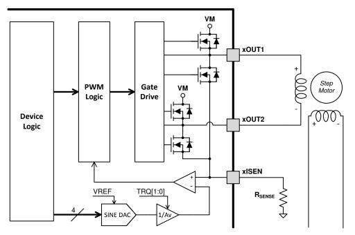
Figure 13. PWM Motor Driver Block Diagram
