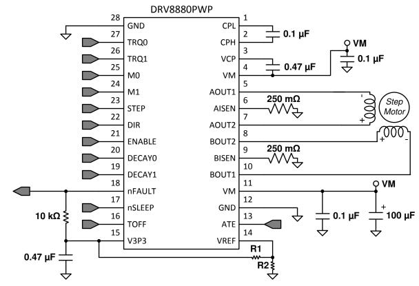
Figure 28. Typical Application Schematic
