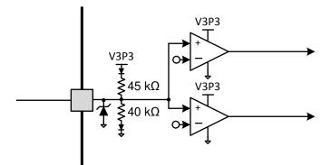
Figure 24. Tri-level Input Pin Diagram
