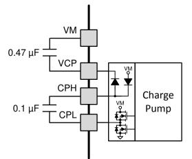
Figure 21. Charge Pump Diagram
