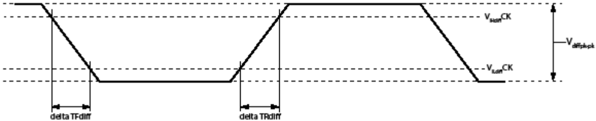
Figure 9 — Differential Input Slew Rate Definition for CK_t, CK_c
