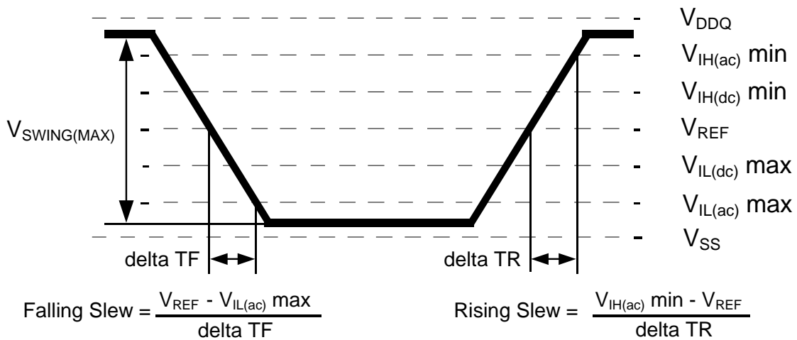
< Figure : AC Input Test Signal Waveform >
