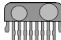
TFDH6542 Side View Through Hole SIL
