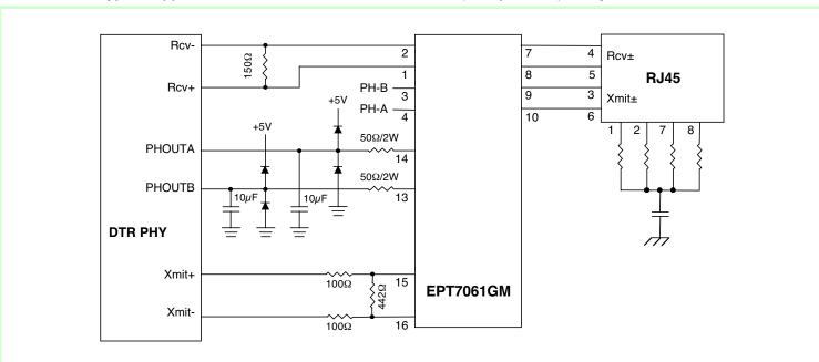
Notes: 1. Pins 3 & 4 are left unconnected. Applications vary. Your system may have a phantom drive return detection circuit needing pins 3 & 4 to be connected separately.
