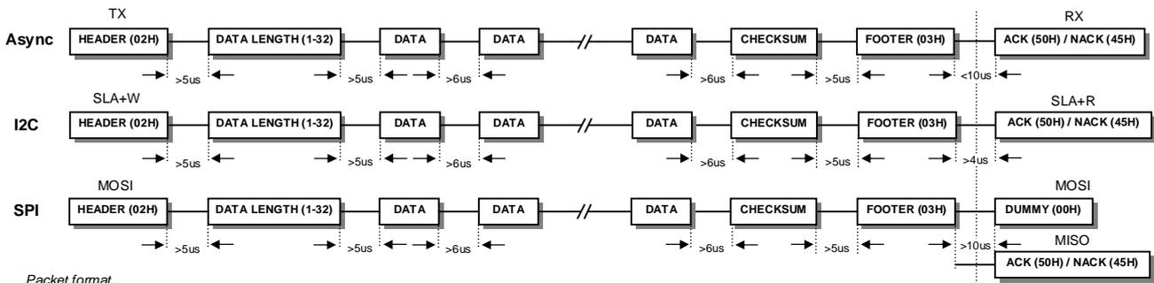
Example asynchronous packet transfer: -
