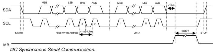
The SCL and SDA lines are internally pulled up with 10K resistors.
