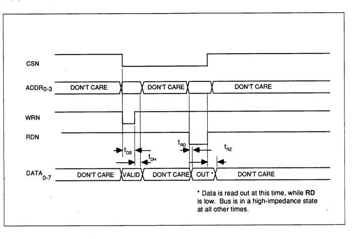
**A.C. CHARACTERISTICS** (Operating Conditions:  $V_{DO}$ =5.0 volts ± 5%,  $V_{SS}$ =0 volts,  $T_a$ =0° to 70°C)
