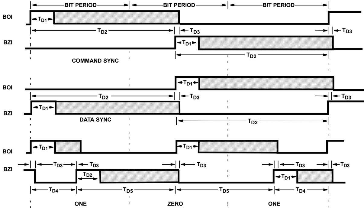
NOTE: BIPOLAR ONE IN = 0, BIPOLAR ZERO IN = 1, FOR NEXT DIAGRAMS.
