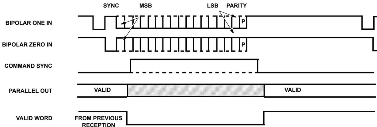
FIGURE 5. DECODER TIMING
