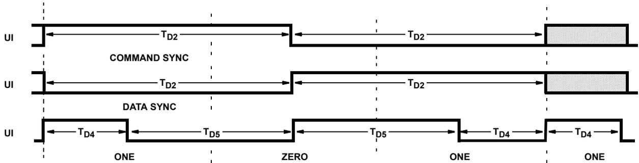
FIGURE 11. DECODER TIMING
