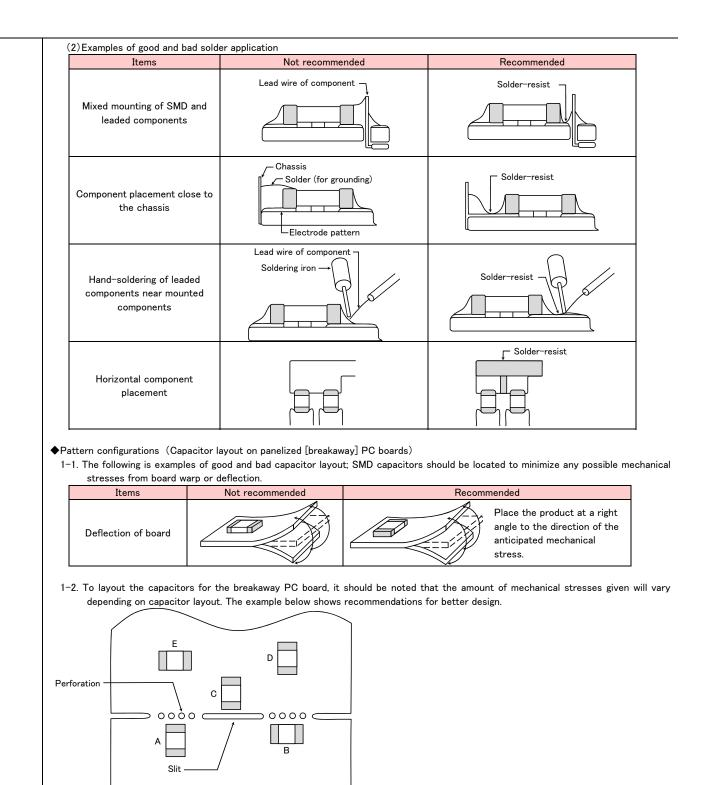
1-3. When breaking PC boards along their perforations, the amount of mechanical stress on the capacitors can vary according to the method used. The following methods are listed in order from least stressful to most stressful: push-back, slit, V-grooving, and perforation. Thus, any ideal SMD capacitor layout must also consider the PCB splitting procedure.
