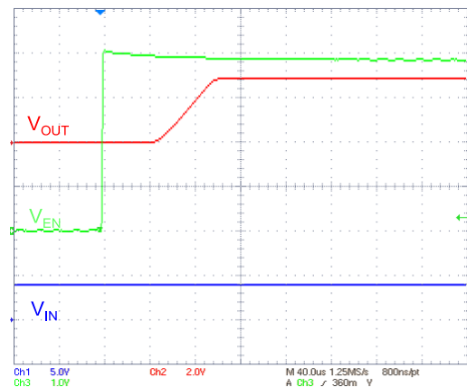
Figure 27: Enable transient ( I_{OUT} = 250 mA)
