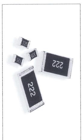
resistive element is screen printed and fired and the passivation layer added. Each resistor is trimmed to tolerance by laser. The pre-scribed tile is broken into strips, the end plating is fired on and the strips broken into individual components. Final termination is made by electroplating. Precious metal terminations are screen printed onto a ceramic base and fired. The
