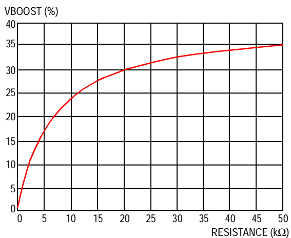
Figure 11. Voltage Boost as a Function of the RBOOST Resistor
