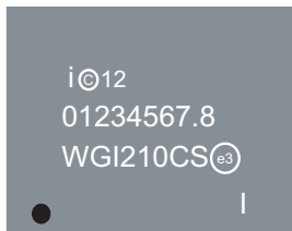
Figure 1-5. I210 Production Top Marking Example (Automotive Industrial Temperature Fiber)
