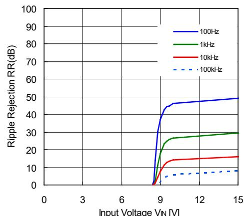
**7) Ripple Rejection vs. Frequency ( $T_a = 25^\circ\text{C}$ , Ripple = 0.5 Vpp)**
