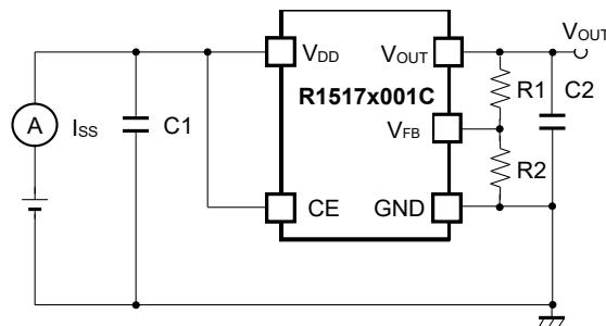
**R1517x001C Supply Current Test Circuit**
