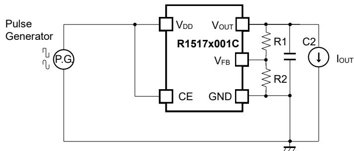
**R1517x001C Ripple Rejection Test Circuit**
