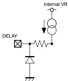
**DELAY Pin (R1517xxxxE/F)**
