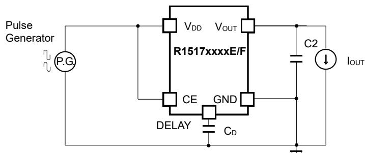
**R1517xxxxE/F Ripple Rejection Test Circuit**
