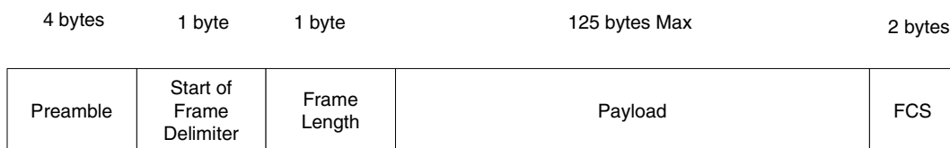
Figure 3. MC13191 Packet Structure
