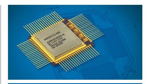
The Honeywell 16 Megabit radiation hardened low power non-volatile Magneto-Resistive Random Access Memory (MRAM) offers high performance and is designed for space and military applications. The part can be configured as either a 2,097,152 word x 8-bit or a 1,048,576 word x 16 bit MRAM through an external pin setting.
