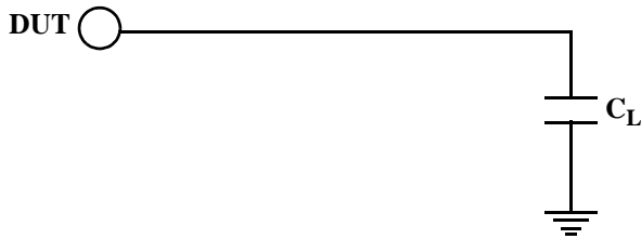
Figure 10. Output Test Load Circuit for LOCK and Dynamic Power Supply Current Measurements
