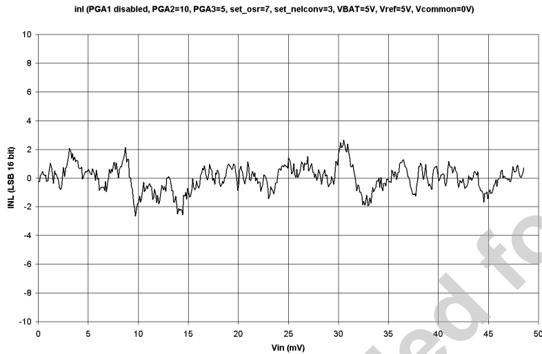
Figure 17-14. Integral non-linearity of the ADC and gain of 50 (PGA1 disabled, PGA2=10, PGA3=5, reference voltage of 5V)
