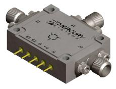
The Mercury Systems PIN diode SP2T switch family spans the frequency range of 0.5 – 18 GHz. It offers high performance and an integrated high speed driver controlled by TTL or CMOS signals. This switch will maintain high performance as a drop in device for system or subsystem requirements. The Mercury Systems family of high performance switches is available in military or non military versions, hermetic and non-hermetic.
