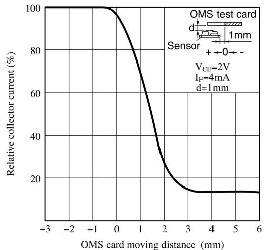
**Fig.13 Detecting Position Characteristics (2)**
