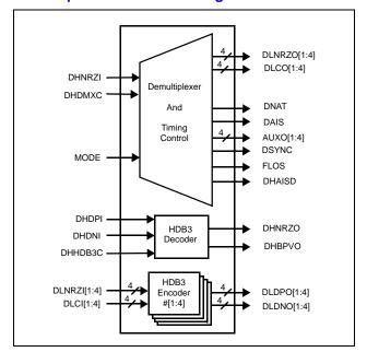
Figure 6. Demultiplexer Side Block Diagram
