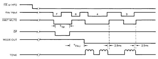
Trsh: flash time 96 or 640 ms (F1 or F2 respectively) for UM91215 flash time 297 or 640 ms (F1 or F2 respectively) for UM91214
