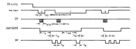
Td: Delay time of Key valid to dialing signal out, typically 0ms
