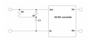
D1 = Hold-up mode diode C1 = Hold-up capacitor
