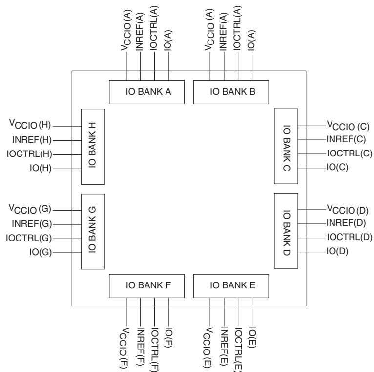
Figure 46: QL5842 I/O Banks with Relevant Pins
