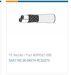
Twisted Pair Cable, MIL-DTL-27500, 600VAC Voltage Rating, 20AWG Wire Size, Operating Temperature Range -65 – 200 °C
