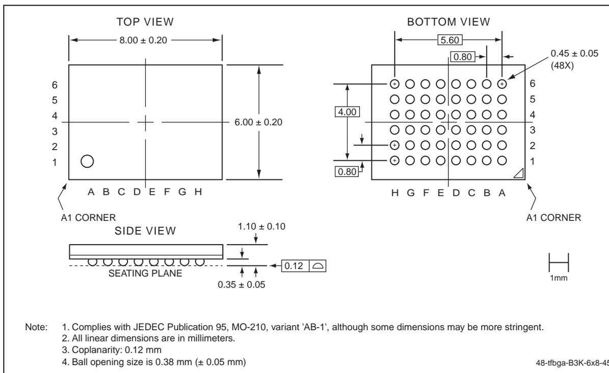
**Figure 24:** 48-Ball Very-Very-Thin-Profile, Fine-Pitch Ball Grid Array (WFBGA)
