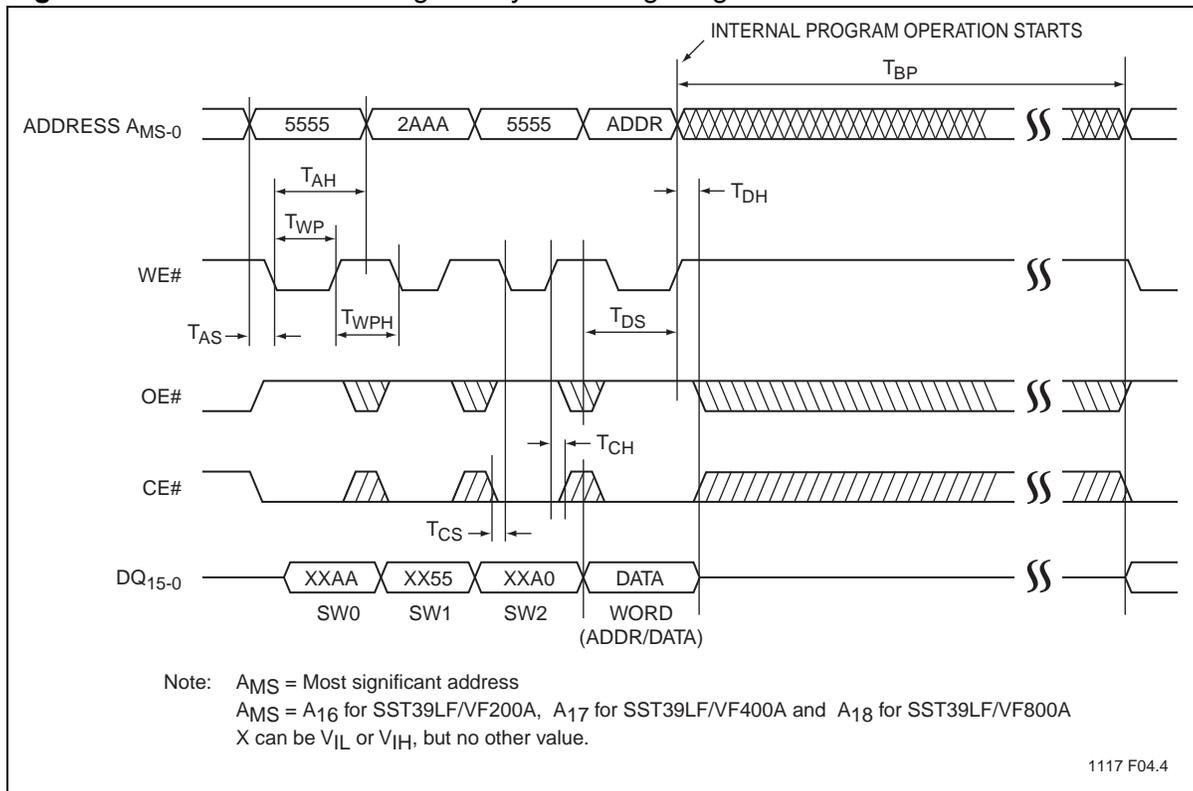
**Figure 7: CE# Controlled Program Cycle Timing Diagram**
