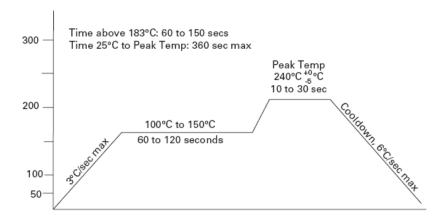
\*Note: These profiles were used during the qualification testing of the product and therefore represent worst case conditions. They are not recommended for use by the customer in the actual assembly of these parts.
