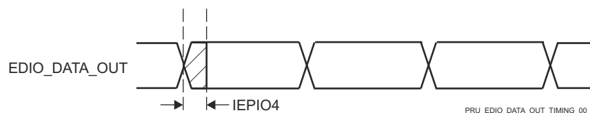
Figure 7-111. PRUSS IEP Digital IOs Timing Requirements
