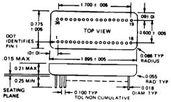
PACKAGE IS KOVAR WITH ELECTROLESS NICKEL PLATING PINS ARE KOVAR WITH GOLD PLATING (50 µINCH MIN) CASE IS ELECTRICALLY FLOATING
