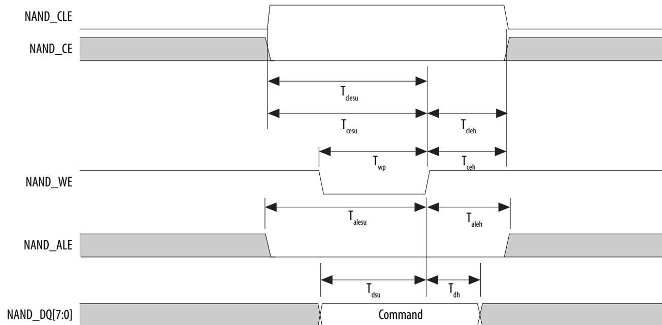
Figure 15: NAND Address Latch Timing Diagram
