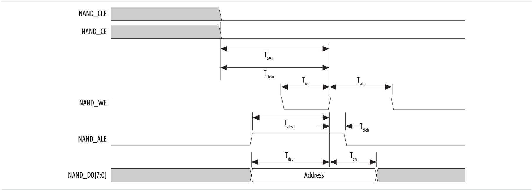
Figure 16: NAND Data Write Timing Diagram
