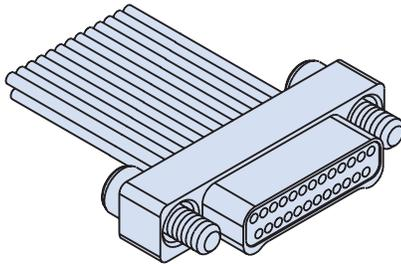
**Nanominiature Connectors with Insulated Wire** feature gold alloy TwistPin contacts. Contacts are precision-crimped to insulated, stranded wire. These nanominiature connectors offer premium performance and reliability for demanding applications. Contact spacing is .025 inches. 1 amp current rating, DWV rating 250 volts AC. Wire gages #30 and #32 AWG.
