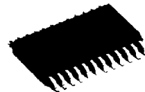
Outline 24P2W-A(FP) 1.27mm pitch 450mil SOP (8.4mm × 15.0mm × 2.0mm)
