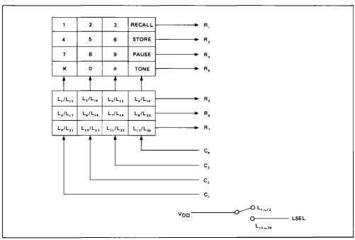
A 7 x 4 single contact keyboard shall be used.  $L_1/L_{13} \sim L_{12}/L_{24}$  are one touch memory recall keys. By connecting or disconnecting LSEL to/from V<sub>DD</sub>, two telephone numbers can be assigned for each key. So, the 24 numbers in total can be recalled by single key operation.
