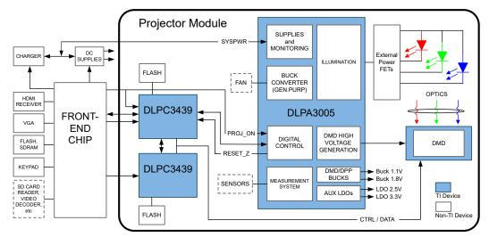
Figure 8-1. Typical Setup Using DLPA3005
