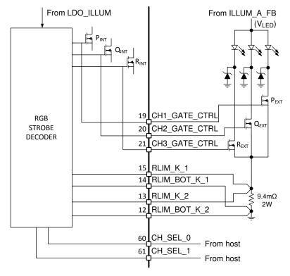
Figure 7-6. Switch Connection for a Common-Anode LED Assembly
