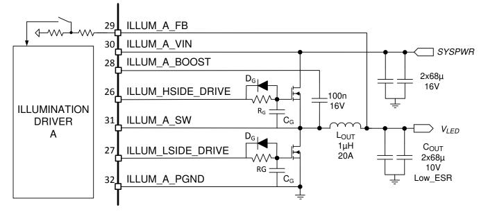
Figure 7-4. Typical Illumination Driver Configuration
