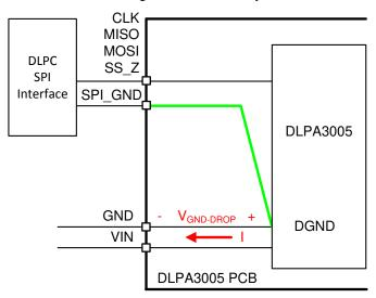
Figure 10-2. SPI Connections
