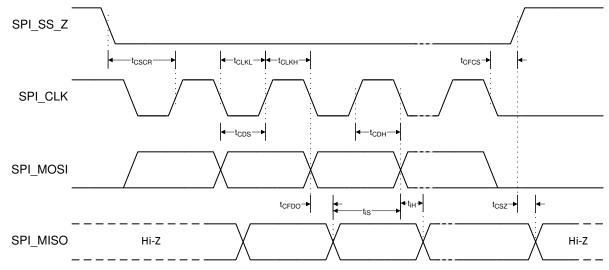
Figure 7-21. SPI Timing Diagram
