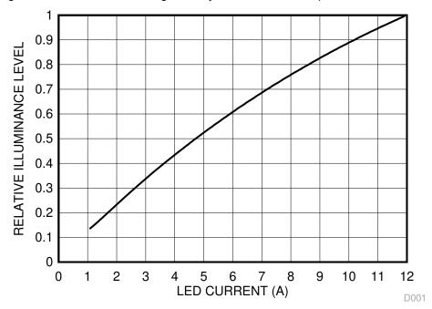
Figure 8-2. Luminance vs LED Current
