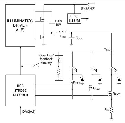
Figure 7-2. Illumination Control Loop
