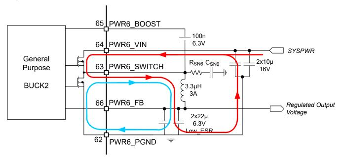
Figure 10-1. High AC Current Paths in a Buck Converter
