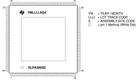
Figure 11-1. Package Marking DLPA3005 (Top View)
