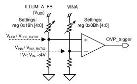
Figure 7-9. Ratio Metric OVP
