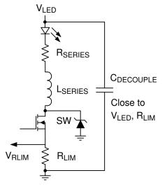
Figure 10-3. Parasitic Inductance (L<sub>Series</sub>) and Resistance (R<sub>series</sub>) in Series with LED
